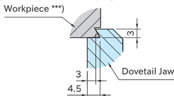
\*\*\*) Preparation of dovetail groove on workpieces is required.
