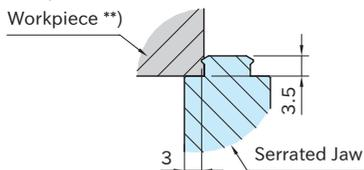
\*\*\*) Workpiece hardness should be HRC38 or less for use of serrated jaw.
