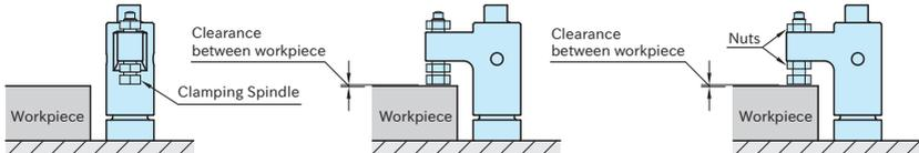
1. Apply air to the unclamping port with an air blow gun to move the clamp to unclamping position.
