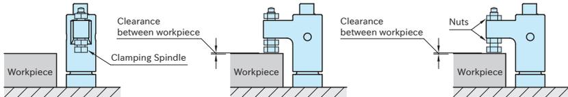
1. Apply air to the unclamping port with an air blow gun to move the clamp to unclamping position.
