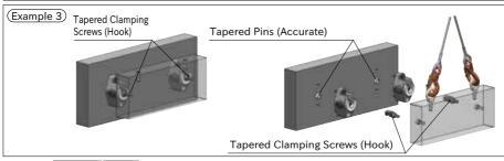
Note: Use CP166-H CP166 Clamping Screws when locating of workpiece is not necessary.
